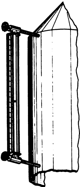
Figure V-8. Rectifying Column Sight-Glass
