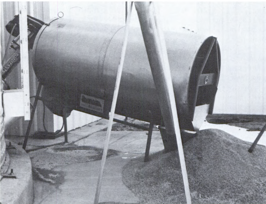
A grain cleaner prepares the milo at the Shroder Farms Alcohol Plant in Campo, Colorado. Forced air and rotary motion remove loose hulls, weeds, rocks, and dirt.
