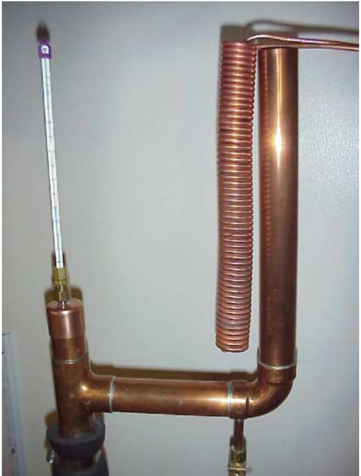
Still Head with Heat Exchanger Revealed
